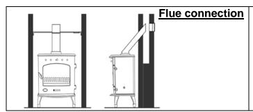
Attach the flue outlet to the stove with the screws and nuts provided. Use a steel closure Attach the flue outlet to the stove with the screws and nuts provided. Use a steel closure plate to seal off the chimney; a cleaning door must be fitted into the plate, and a steel sealing collar must be used to fit the flue into the steel plate. Seal all joins with fire cement.
